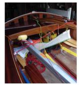
Most other kit that is normally carried aboard while sailing can travel in its usual position without special preparation. Making sure that the **spinnaker pole** is either clipped or tied so it can't move around.
