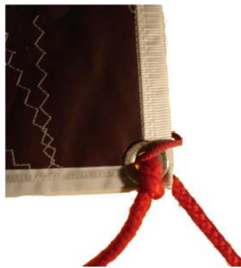
Simple overhand knot inside the cringle is sufficient to secure sheets (in this example it is pulled out to one side for the photo). Also shows loop of light line for hooking in jibstick or spinnaker pole.
