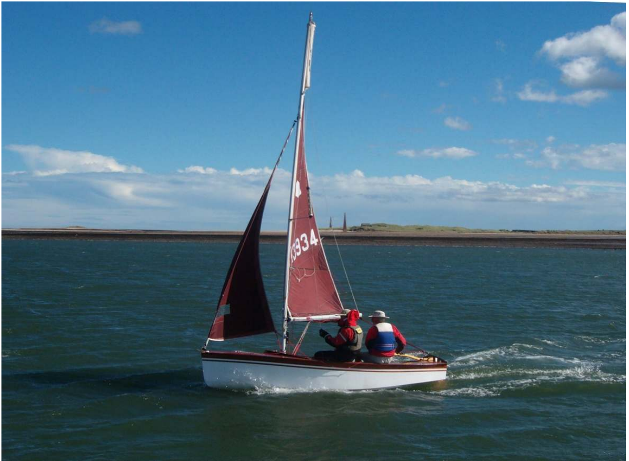
The writer's Series 2 boat "A Capella" in blustery conditions in Holy Island Sound, 2010. Genoa clew is cut a little higher than standard, to give acceptable sheeting angle when reefed. Don't be misled by the flat water, it is sheltered by drying banks all round, and conditions were indeed seriously blustery.
