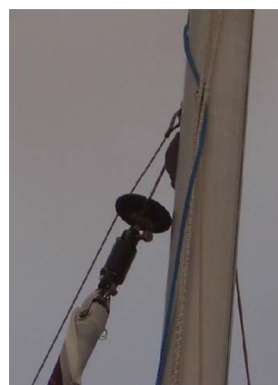
Preventer disk above top swivel keeps forestay clear of head of sail
