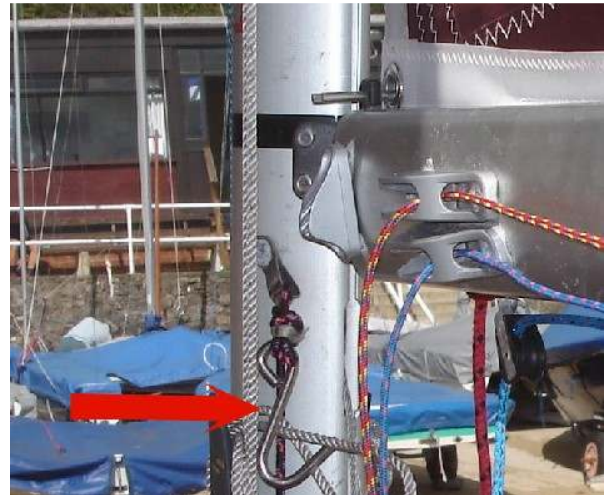
Reefing lines led forward to near mast. Also showing downhaul (arrowed), led through fairlead
