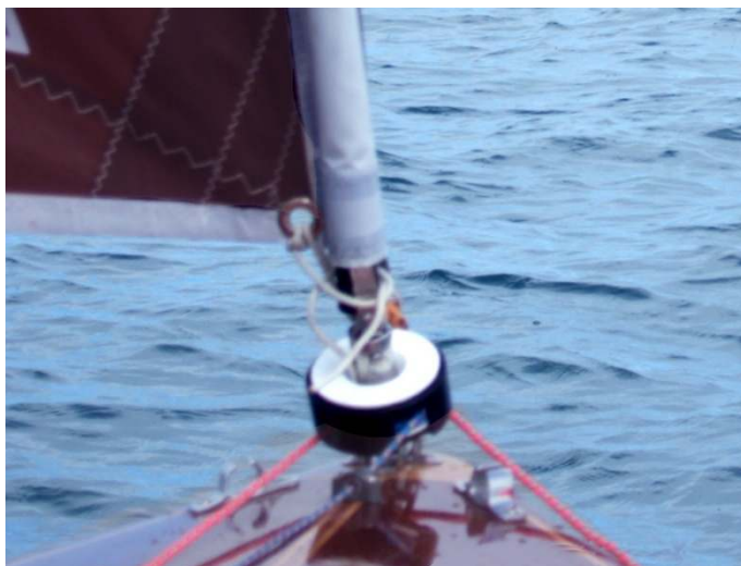
Sea-Sure enclosed reefing/furling drum, also showing special luff pocket with reefing spar inside it.
