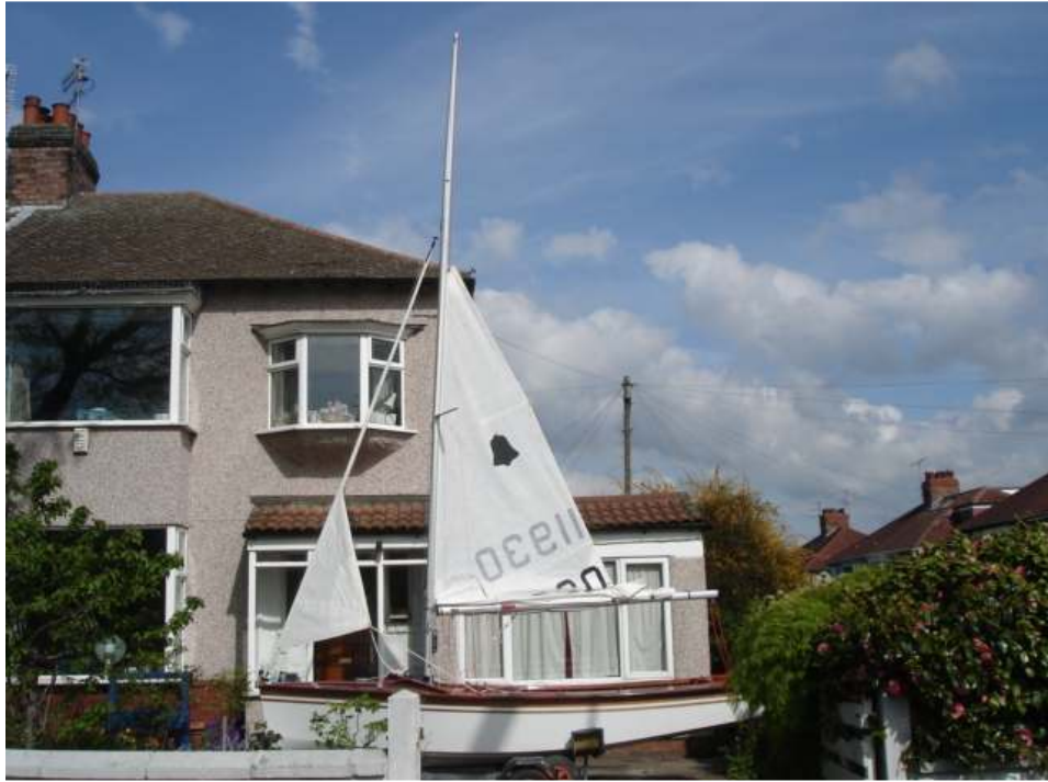
(Above and below): Second reef in main, and genoa reefed to a spitfire jib size. This is a very snug rig indeed, and the writer has used it in Force 7/8.
