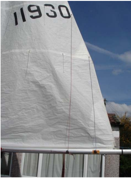
Reefing lines in place, 3 mm Dyneema or similar. These are rigged on all occasions when the boat is sailed.
