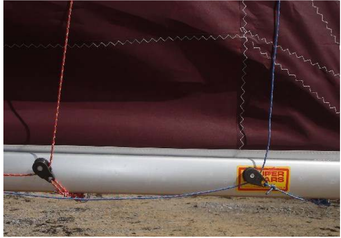
This photo shows the blocks, with plastic cheeks, on lanyards, secured to boom sliders; pre-set the slider positions and lengths of lanyard to suit the sail.
