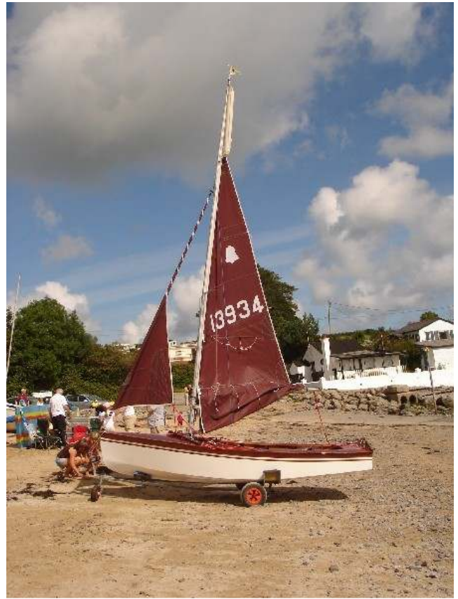
Reefing procedure; STEP 2 Slack off halyard and pull luff downwards. The boat is immediately sailable in this condition.
