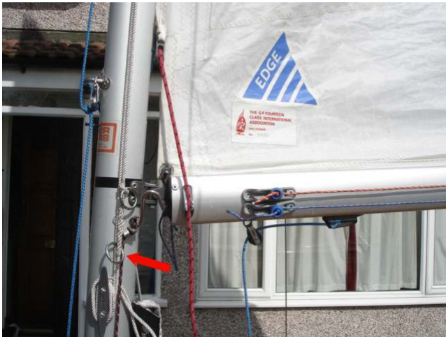
Reefing lines led forward to near mast. Also showing downhaul (arrowed), led through fairlead
