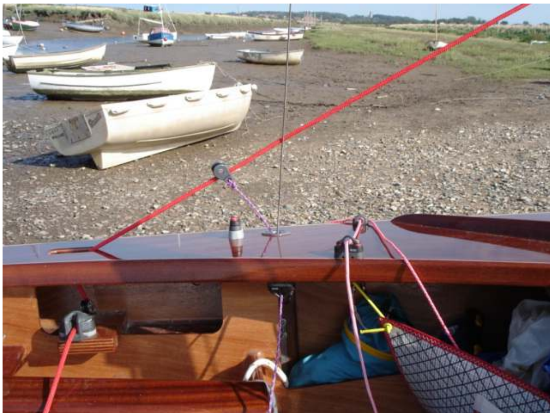
Block running free, but light tension on line. An artificial photograph, just to illustrate the system; one would never sail with it in this position.
