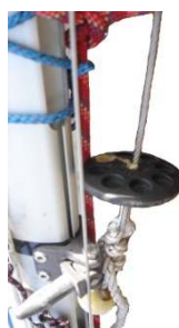
Preventer disk on halyard. (Mast stripped for transit)
