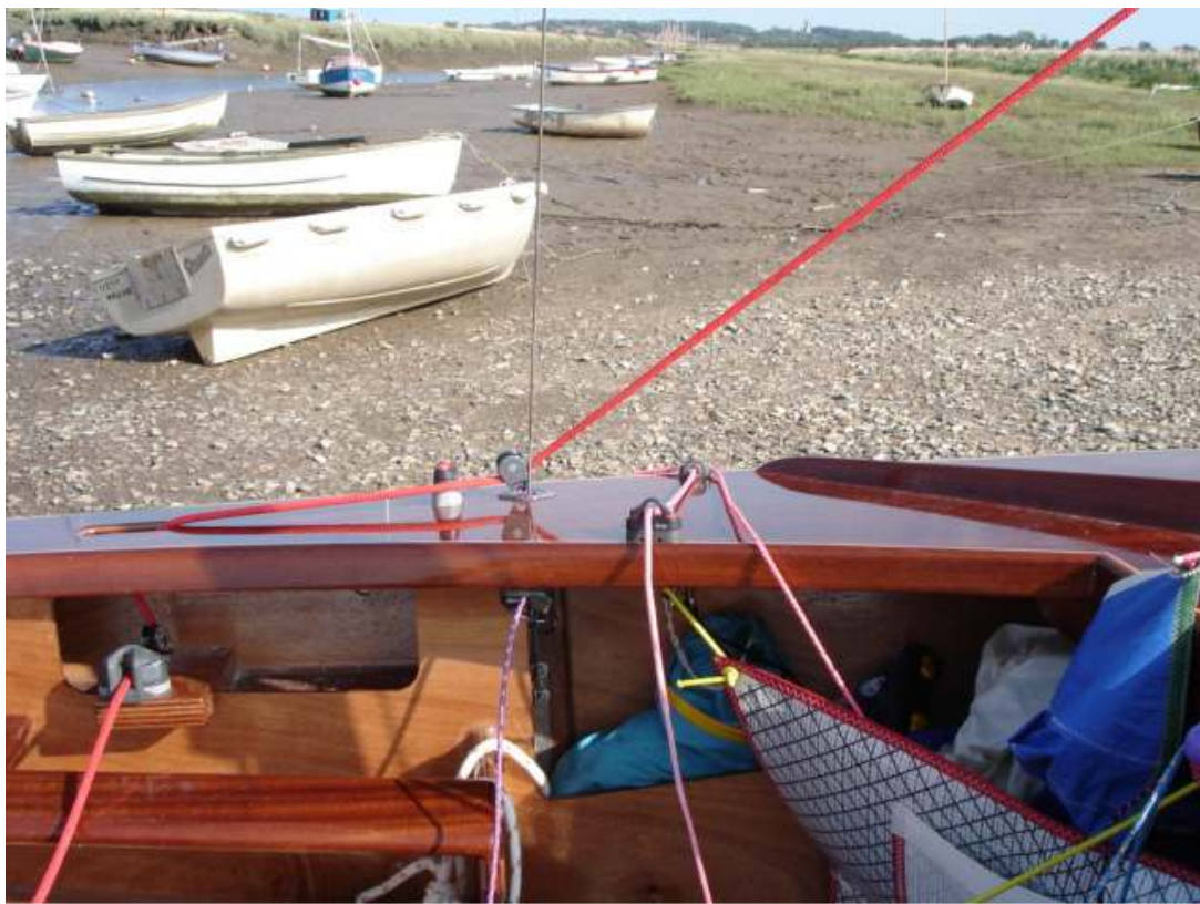
Partial solution; block pulled down, to improve sheeting angle
