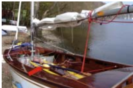
Spinnaker pole pressed into service to support the inboard side of the bed base.
