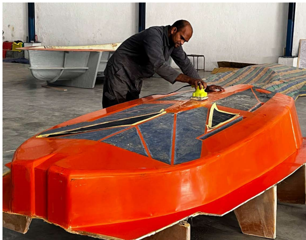
Inner Tray-The mold for the inner tray has been fabricated with a special nonslip pattern that will be transferred onto the production inner tray
