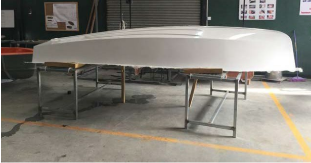
The Hull follows the exact shape of the Duffin Hull used as the plug
