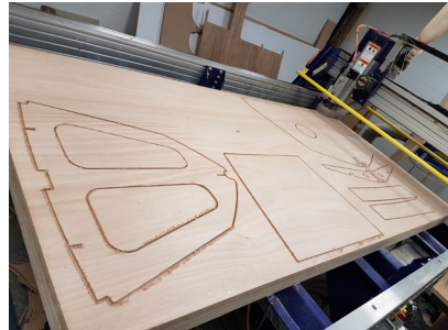
Panels CNC cut
