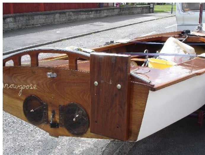
Set up for purposes of the photo only; lower pair of coach bolts would of course be fitted in normal use, but I was a little lazy in setting up this photo shoot!
